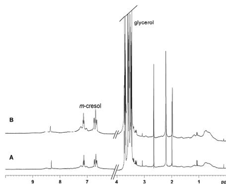
Figure 6. <sup>1</sup>H NMR water presaturation spectra (watergate) of ACTRAPID (A) and ACTRAPID after 6 h of irradiation (B) at 0.1 mM concentration in D<sub>2</sub>O/H<sub>2</sub>O 10/90, 298 K.
