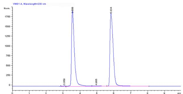
Figure 3. Typical RP-HPLC chromatogram of Actrapid $^\text{TM}$  showing two main peaks of UV absorbance at 230 nm.
